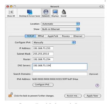
Temporary Network Configuration for Connection with Firewall Defaults - Mac OS X
